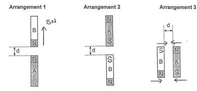
In Arrangement 1, Magnet B experiences a repulsive force of 5 N upwards.
