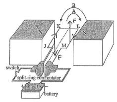
a) Does the coil rotate in the direction shown as **A** or in the direction shown as **B** (see diagram)? Explain how you decided.
