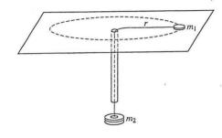
An experiment is performed using the apparatus above. A small disk of mass  $m_1$  on a frictionless table is attached to one end of a string. The string passes through a hole in the table and an attached narrow, vertical plastic tube. An object of mass  $m_2$  is hung at the other end of the string.
