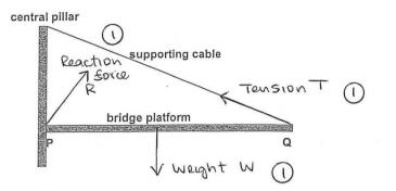
(a) The structure is in equilibrium even though there are **three** forces acting on it. **Draw** and **label** these three forces on the diagram.
